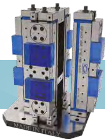
FMS vise tower made of 4 vises Art.865 vertically mounted through spacers with floating movable jaws and intermediate fixed jaw.
